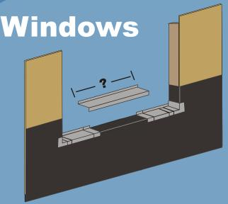
1. Install lower course of housewrap. Place left & right corners tight against framing. Measure center section and cut if necessary maintaining 1 ½" overlap at glue joints. Center section must fit within recessed areas of corner pieces.
