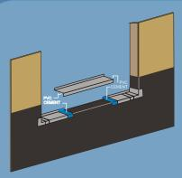
2. Apply PVC cement to the recessed areas of the corner pieces and the underside of the center section where it overlaps the recessed areas. Hold or clamp pieces together long enough to ensure a complete bond.
