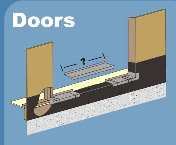
1. Install lower course of housewrap. Place left & right corners tight against framing. Measure center section and cut if necessary maintaining 1 ½" overlap at glue joints. Center section must fit within recessed areas of corner pieces.
