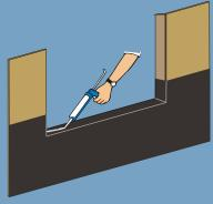
3. Remove pan and apply caulking where the pan will contact the framing. Set pan in caulking.
