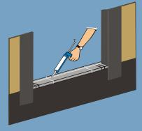
4. Apply caulking to interior edge of pan to seal window frame/door sill to pan. Apply caulking to glue joints for added protection. Adhere flexible flashing to sides of opening, wrapping around from sheathing to studs and shingle over and into the sill pan.
